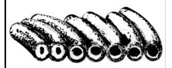
Above is a cross section view showing the progressive liming of coils.
