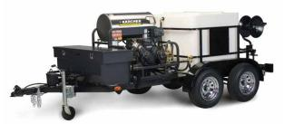
TRK-6000 - shown with options and gas-powered hot water pressure washer; accommodates both gas and dieselpowered pressure washers. Tool box shown is no longer available on this unit.
