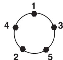
2. Tighten bolts or nuts following sequence at right.
