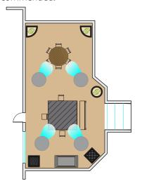
The unit must be placed on level ground to operate correctly. Units create an oval shaped air pattern. Obstacles such as racks and workbenches may interfere with the air flow. An attempt should be made to locate the unit in such a manner that interruption of the air pattern is held to a minimum. Multiple units may be required to cover larger areas.
